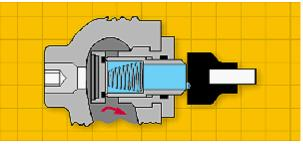
C. Main orifice failed - upstream monitor orifice lock-up. D. V option - vents a small volume of gas to atmosphere through relief valve.
