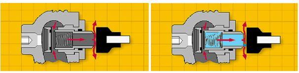
A. Standard regulator and upstream monitor orifice.
